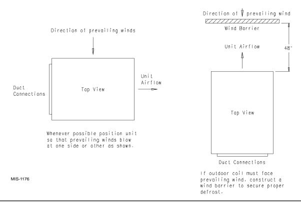
FIGURE 6 SLAB MOUNTING AT GROUND LEVEL (Above 32° F Outside Temperature)
